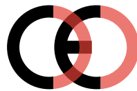
False CE Mark (too close)
