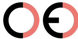
False CE Mark (too far)
